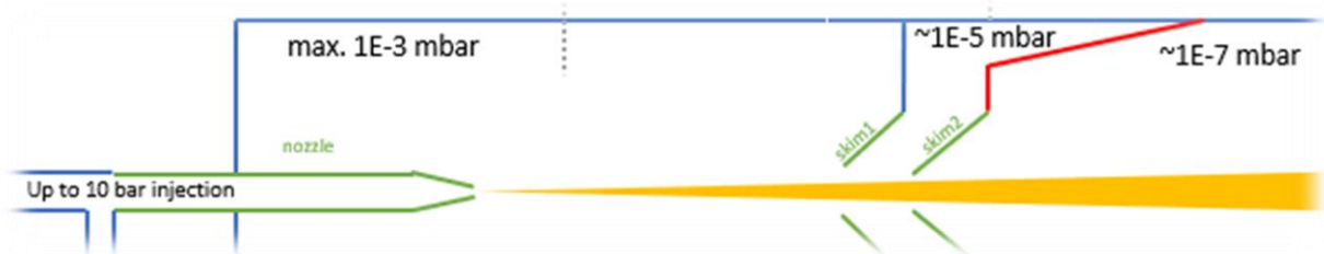
Figure 3: Schematic of BIF monitor only showing the relevant parts to this section.
